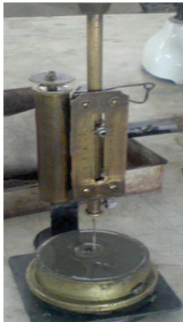
Fig. 3: Vicat apparatus showing measurement of setting time
