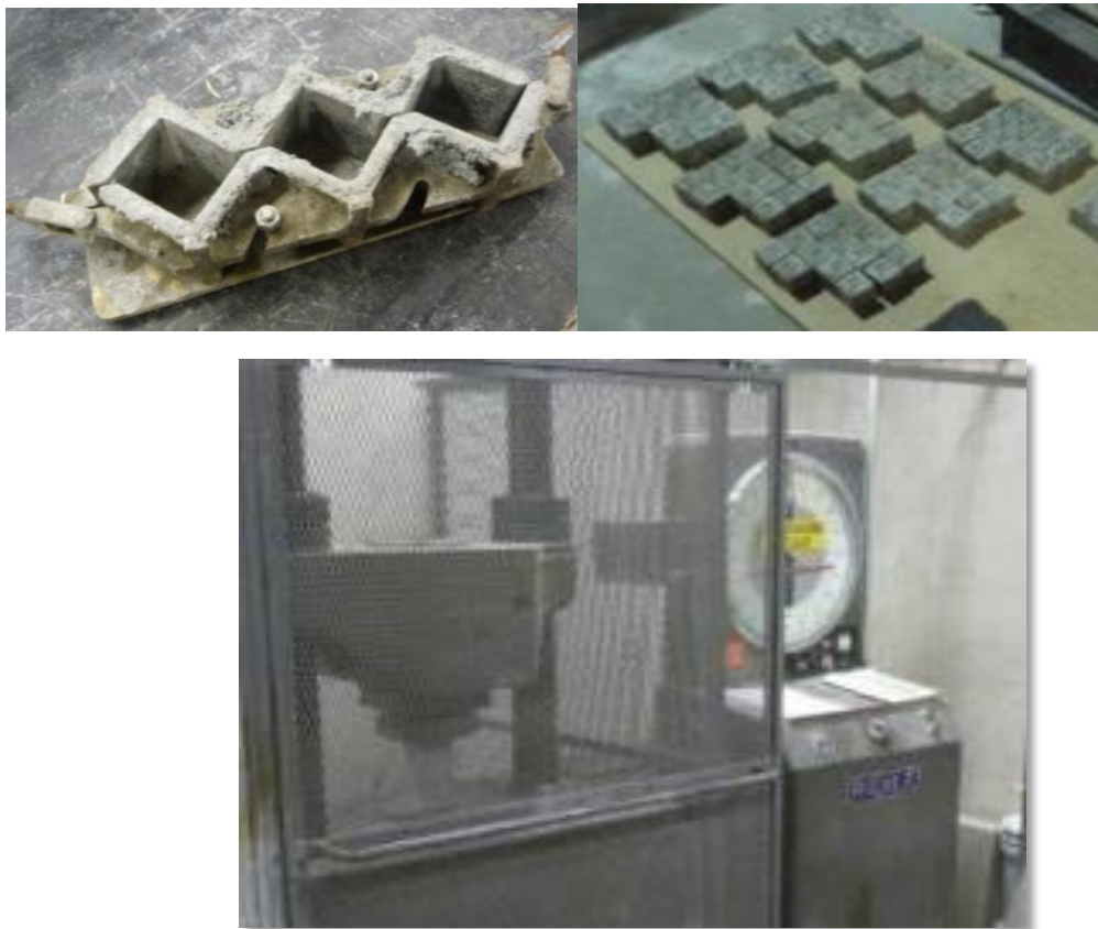
Fig. 2: Cubic mortar specimens and testing for compressive strength
