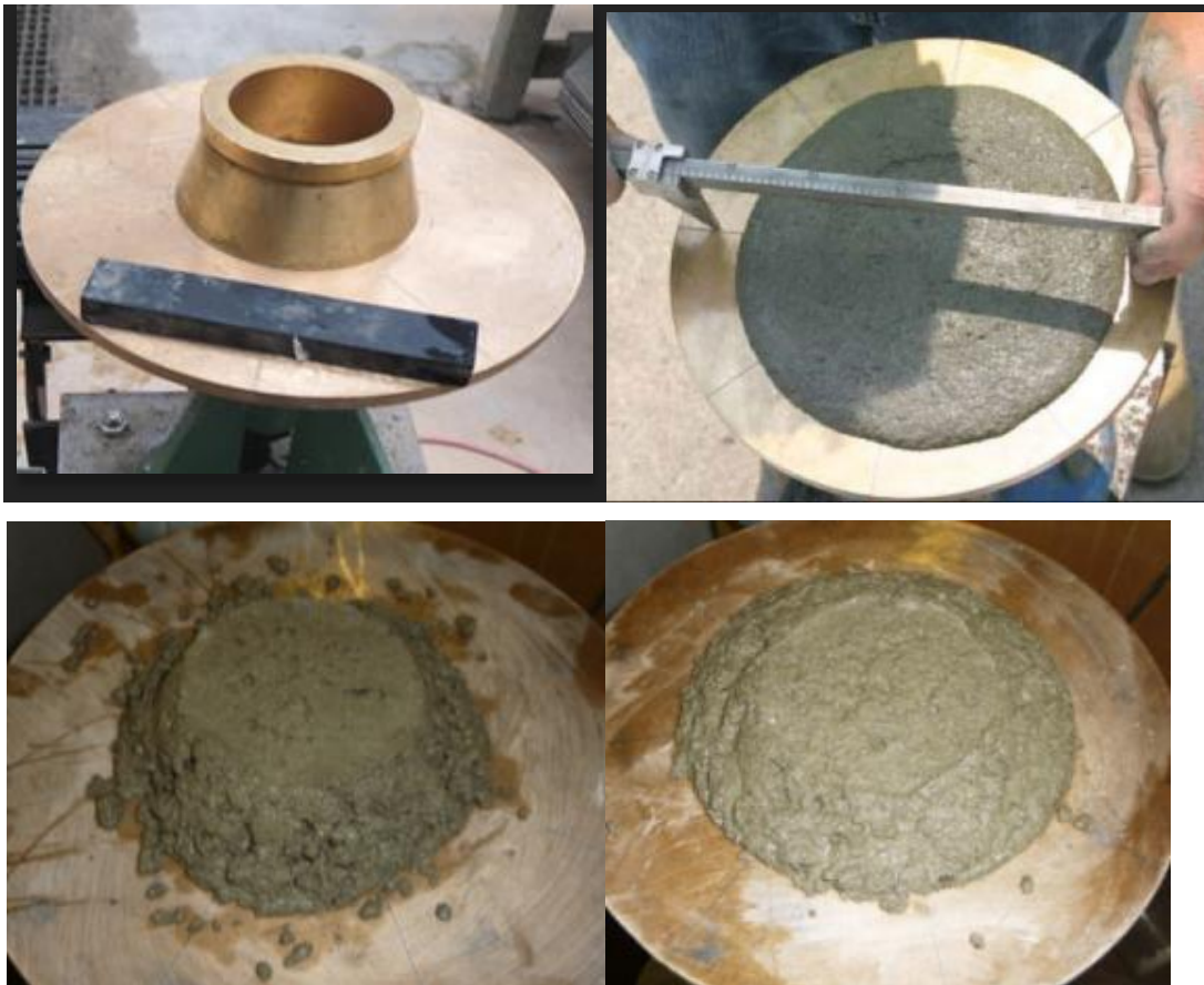
Fig.1: Flow table test set-up, flow and flow measurement
